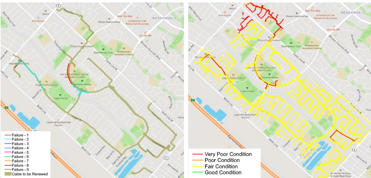
7 Figure 38 – Cable Failures and Condition Maps - Derry Road & Ninth Line
