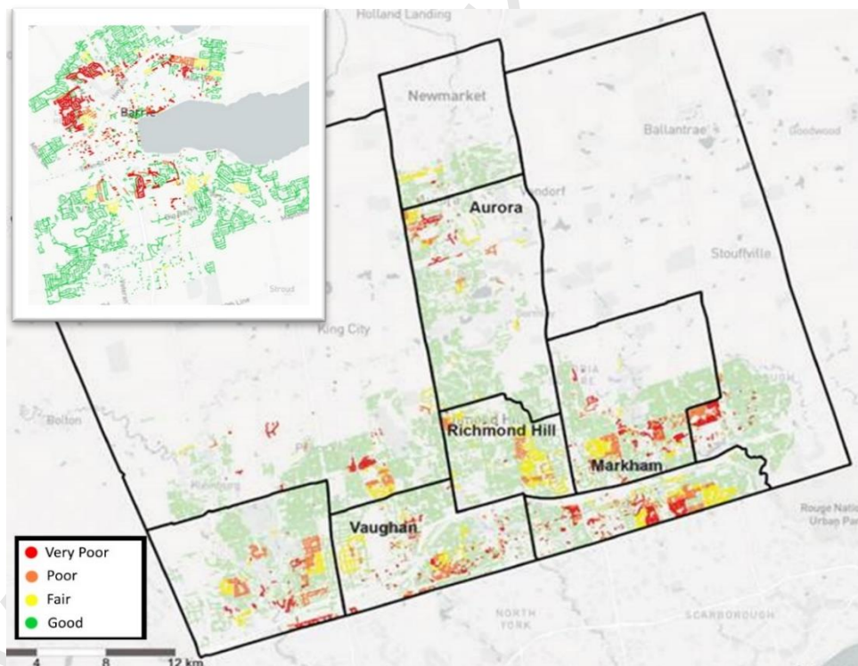
Image: Heat map of cable health condition across former Powerstream service territory (Barrie shown in inset)
