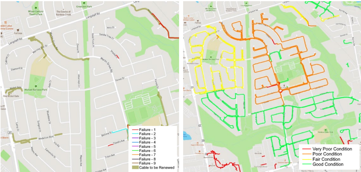
1 Figure 56 – Cable Failures and Condition Maps – Rainbridge Ave
