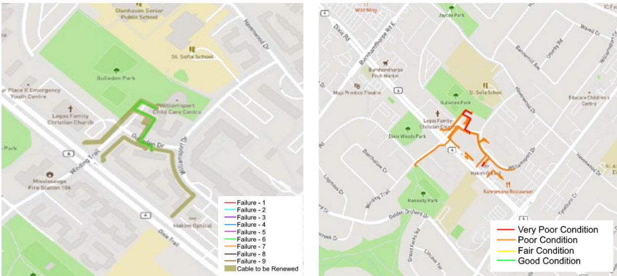
4 Figure 34 – Cable Failures and Condition Maps - Dixie & Winding Trail
