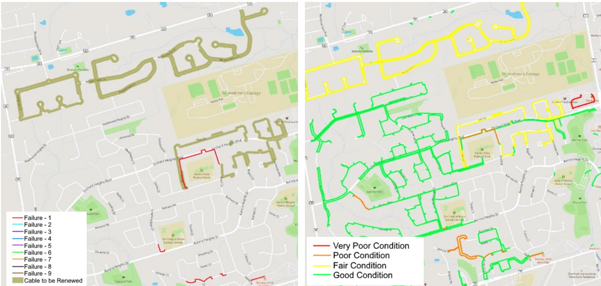
1 Figure 54 – Cable Failures and Condition Maps - Willow Farm Lane Area
