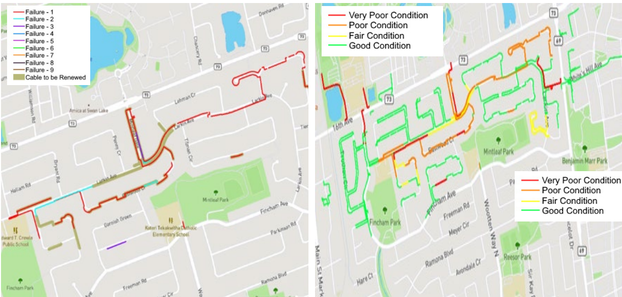
4 Figure 44 – Cable Failures and Condition Maps - Larkin Ave Area
